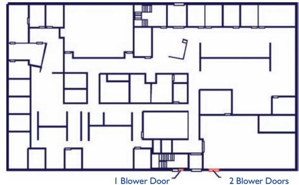
*Figure 1: Building floor plan showing location of blower doors.*
