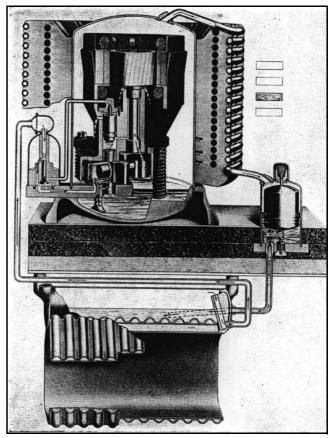
Figure 3: GE DR refrigeration system crossection. (From: Hull, H. 1933. Household Electric Refrigeration)
