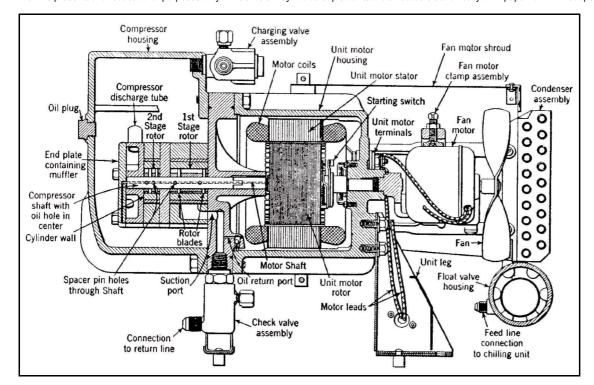
Figure 1: The Holmes refrigerating unit, manufactured in 1928 and 1929, featured a twostage rotary compressor. Like the Allison, the Holmes used a hermetic bladetype rotary compressor with ethyl chloride as the refrigerant. (From: Master Service Manual, #3, "Household refrigeration installation and service")
