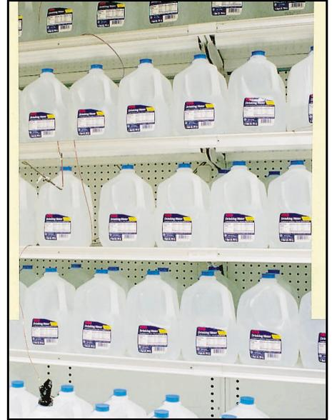
The refrigeration rack (left) provides cooling to the display cases in the controlled environment. Water was used to represent milk during testing.
