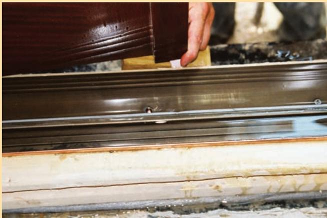
**Testing of exterior door identifying moisture intrusion issue.**
