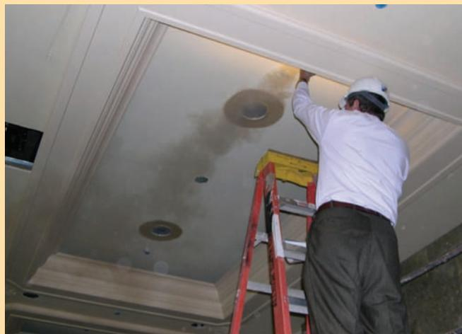
Testing of airflow distribution pattern to assess potential of short-circuiting and adequate distribution.
